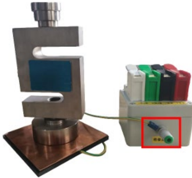
Figure 2: Insulation Measurement Set Up
