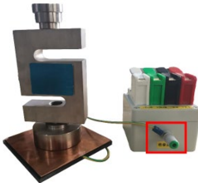
Figure 2: Insulation Measurement Set Up
