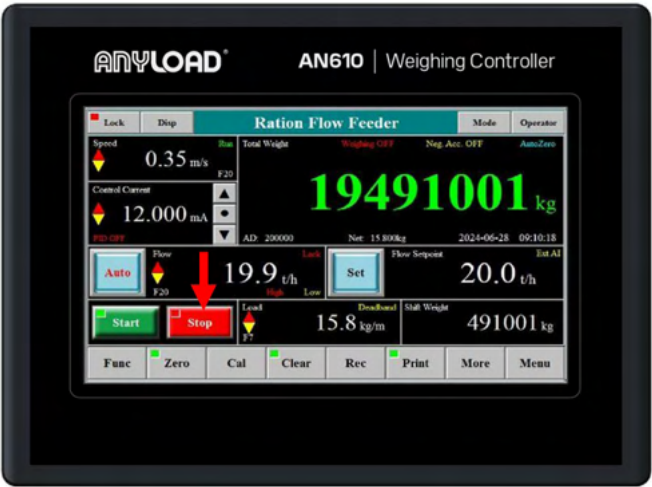
Figure 7-17: Stop Operations Interface Access Button
