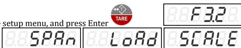
3. Load the scale with the test weight, and press Enter
