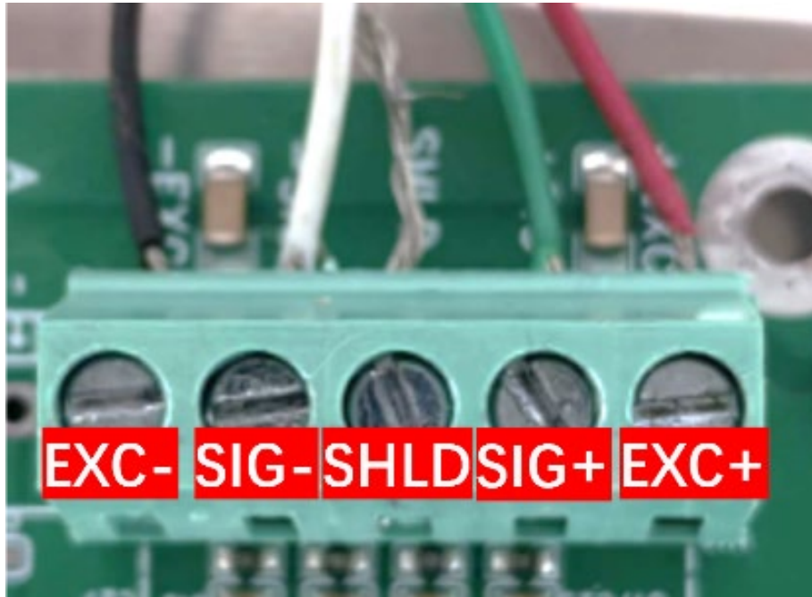
Figure 3-4 Load Cell Wiring Schematic
