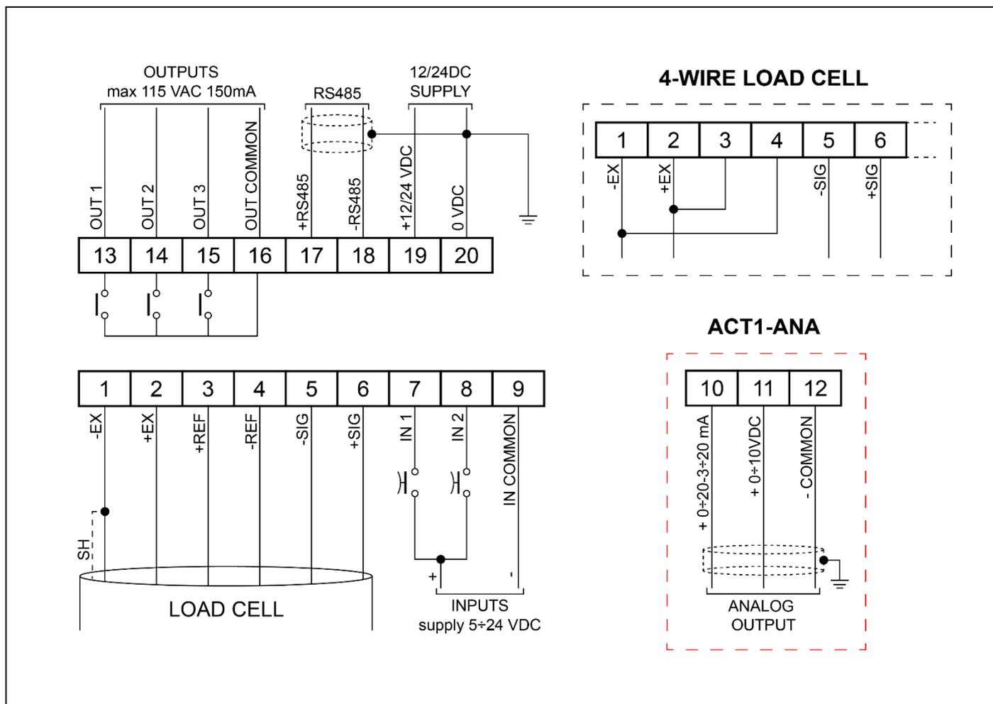
Three outputs, controlled by setpoint values or by a remote device via protocol.
