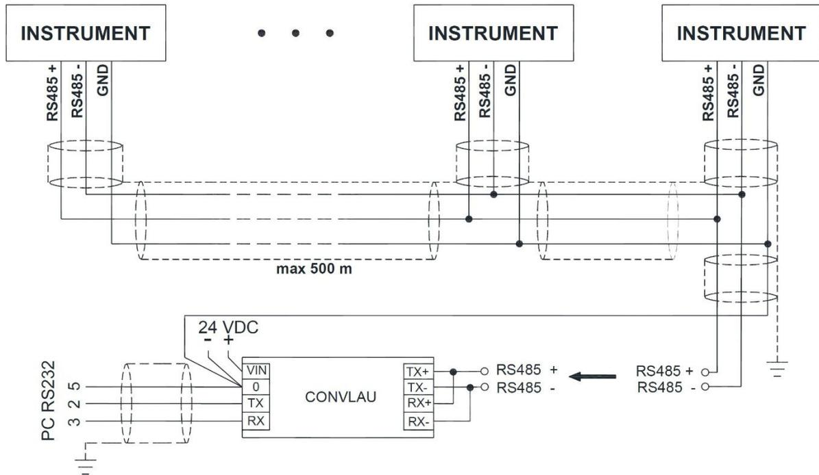
If the RS485 network exceeds 100 meters or if the baud rate is higher than 9600, two terminating resistors are required at both ends of the network.
