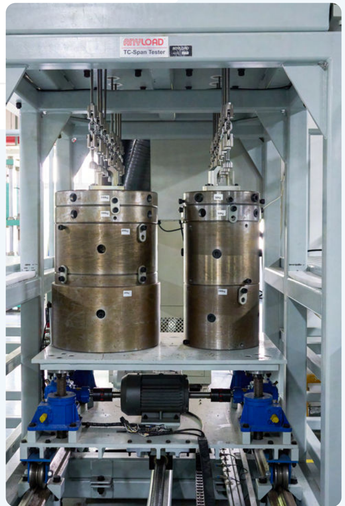
Automated TC Span Test Machine
