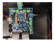
Install the antenna outside the unit at the bottom.
