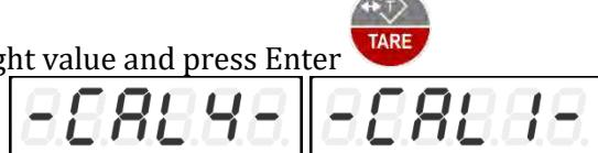
6. Display counts down to span calibration
