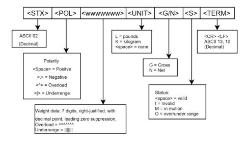
For multi scale and network applications using RS485, there is a similar string format with a dedicated address. This unique address can be set in setup menu. The streaming string also can be set individually for all three communication ports.
