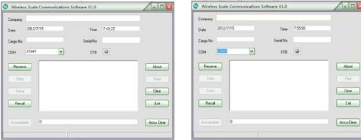
Set the COM port number based on the COM number assigned at device manager.
