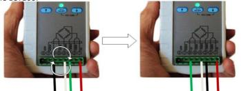
Run the tester using the full testing cycle. The input and output resistance results will be the resistances of a pair of strain gages.
