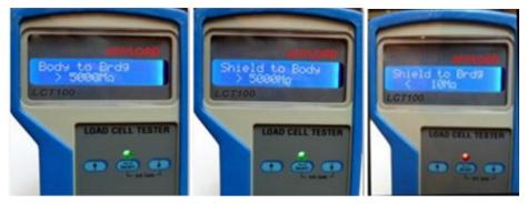
Figure 4 showing the insulation resistance results. The right one is an example of bad result and led turns red
