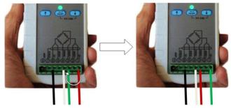
Run the tester using the full testing cycle. The input and output resistance results will be the resistances of the other pair of strain gages.
