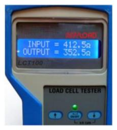
Figure 3 Typical bridge input/output results
