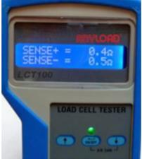
Figure 7 Typical reading when sense lines are OK
