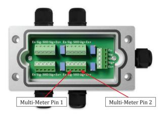
1. Check the resistances of the potentiometers using a multimeter. Place one pin of the multimeter to Sig+ and one pin to Sig- of the load cell terminal to confirm whether they match the factory default settings. Each potentiometer has been adjusted from the factory such that Wi (i =1, 2, 3, 4) is equal to approximately 2.07k $\Omega$  which is the middle of the resistance range from 1.8k $\Omega$  to 2.3k $\Omega$ .
