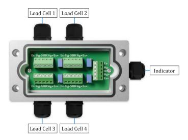
1. Arrange the load cell cable neatly to minimize risk of winding or damage, and insert them through the plastic cable glands. Leave the cable glands grips loose and tighten them securely after wiring. Check the load cell color code listed in the data sheet as it depends on the load cell manufacturer.
