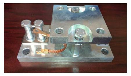
1. Remove the **Top Plate** (Part# 6) and the side **Lock Plate** (Part# 10) by unbolting the fixing screws.
