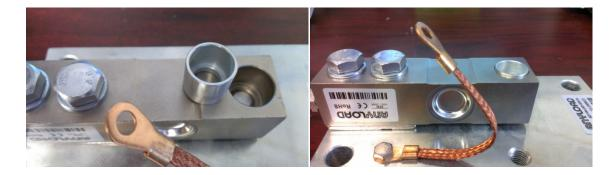
5. Place the Loading Pin (Part# 12) in the Cylinder Ring.
