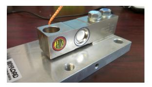
4. Place the **Cylinder Ring** (Part# 13) in the hole of the load cell (only for 563YH load cell) with the thicker edge at the bottom. The **Cylinder Ring** is not necessary for 563YSM3 mount and is not provided with the module.
