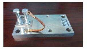
Install the Loading Screw (Part #14) into the load cell threaded-hole until it is at least flush to the load cell recess hole (on the other side of the load cell). All of them should be at the same level. Recommend to use some silicone to fix the Loading Screw position.
