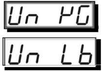
The lb indicator b will light on after **DISPLAY UNIT** switches to lb. The kg indicator kg will light on after **DISPLAY UNIT** switches to kg.
