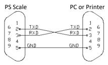
b. Open the serial communication software, for example, "HyperTerminal" in windows. Select the connected portal number "COM" and set the baud rate as 9600bps, the parity bit as "NONE", the data bit as "8Bit", and the stop bit as "1Bit".
