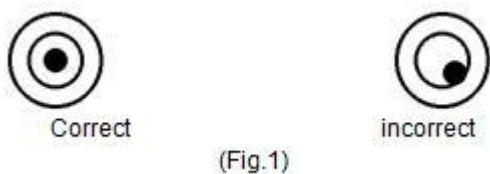
Fig. 1 Correct leveling with the aid of the bubble level and adjusting feet.
